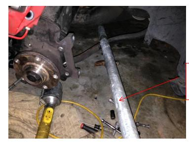
Push down on pry-bar to remove ball joint.
