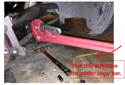
15) With car on ground, tighten up all bolts and nuts to the following:
